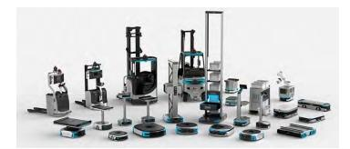
GreyOrange provides a variety of floor robots that can pick up shelves and move parcels around the warehouse (up to 1000kg). They also provide a robot that has a conveyor belt on top to easily pick up and move packages themselves. Each of their robots have different attachments to easily handle different types of packages.
