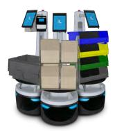
Otto Motors provides floor robots that can scale in size to carry small to large loads (up to 1900kg).
